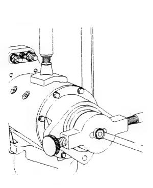
Disassembling control relay and starting-motor solenoid
